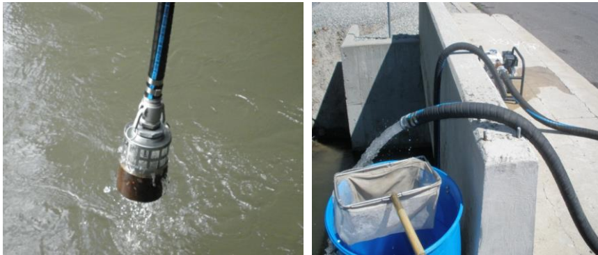
Figure 1. Photographs illustrating the two techniques used for sampling coarse particulate organic matter. With either technique the water was initially filtered through the same net, followed by screening with a 1-mm soil sieve.
