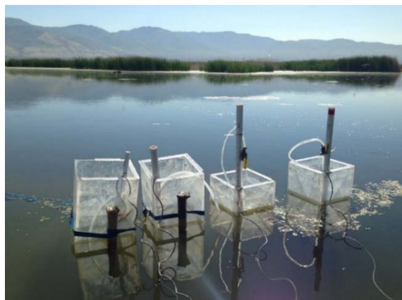
Figure 3: Nutrient flux chambers deployed at site.
