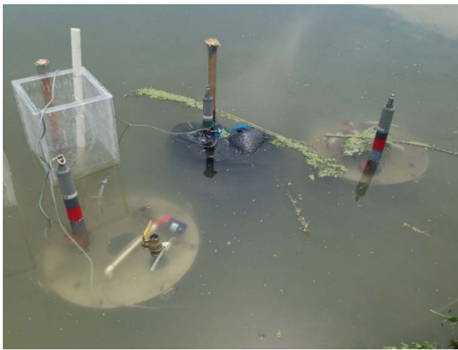
Figure 2: SOD chambers deployed at site.
