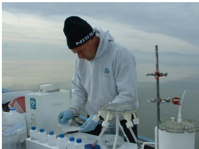
Filtering seston from the watercolumn on Great Salt Lake (photo courtesy Brad Marden)
