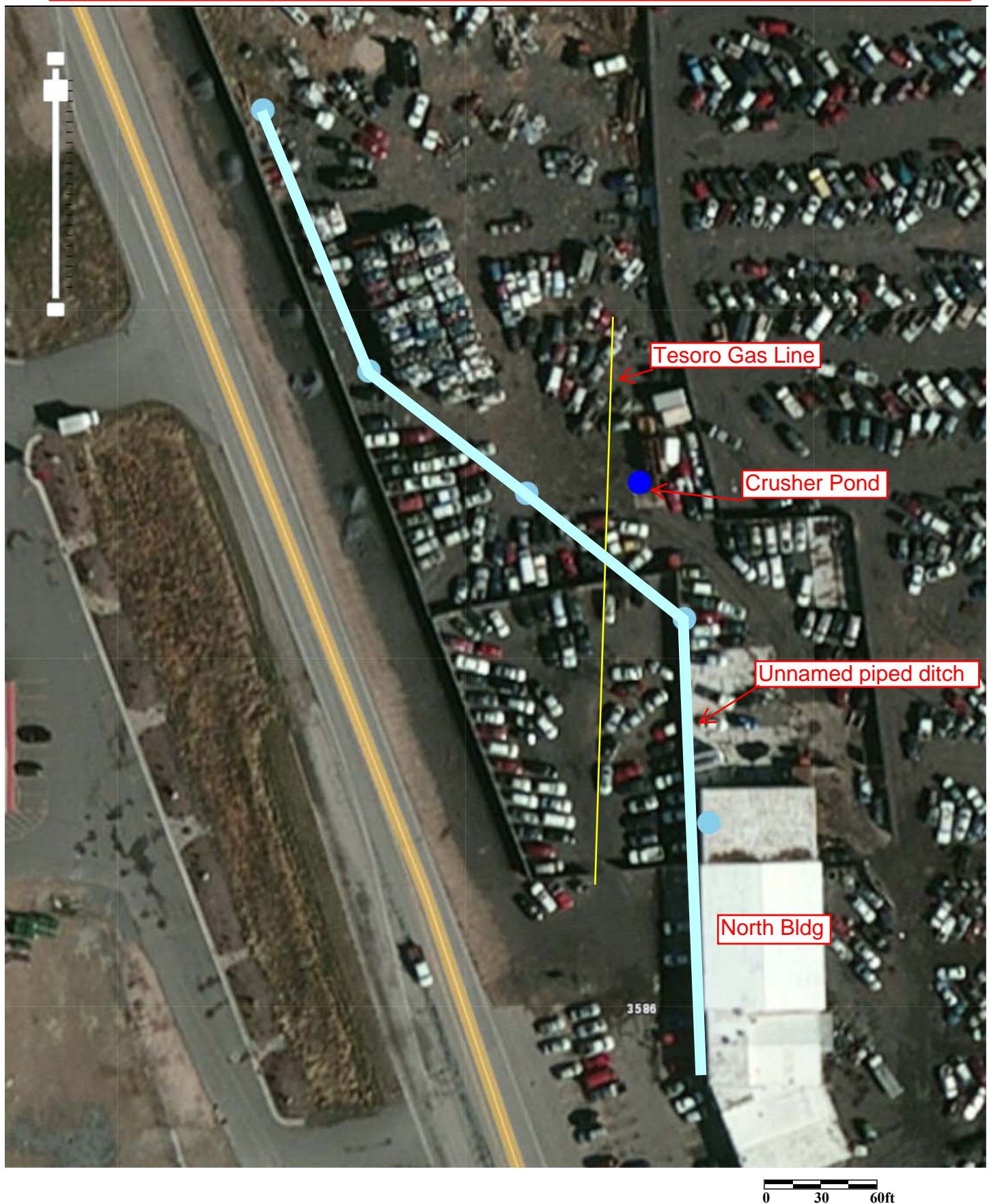
Figure 4, Transwest Pick-A-Part. Utilities buried near the Crusher Pond; utilities outside the west fence are not shown
