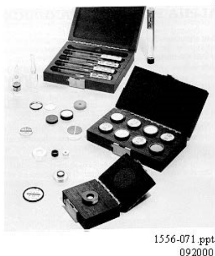
Figure 5-6. Calibration Standards. Certain calibration and reference sources containing americium-241 (Am-241) or Ra-226 can be possessed under a general license authorized in 10 CFR 31.8 by those otherwise specifically licensed.
