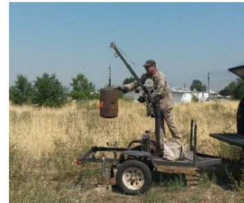
Figure 1. seismic source – 500 lb
