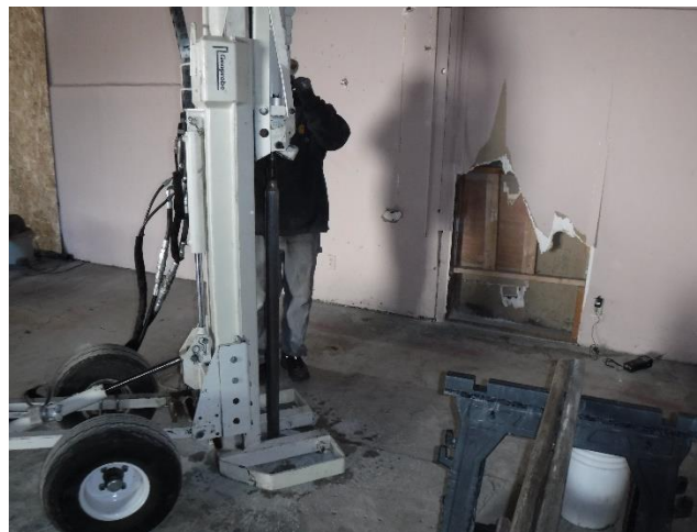
Photo 22 – Typical drilling for confirmation soil sampling activities
