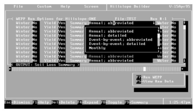
Figure 22. Portion of the WEPP Hillslope Interface run definition table showing the WEPP model output option selection and expanded list for the runoff/erosion summary output type.
