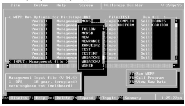
Figure 21. Portion of the WEPP Hillslope Interface run definition table with WEPP input data fields and expanded plant/management file selection list.
