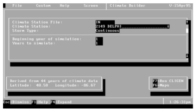
Figure 23. Main Screen of the climate input file builder.
