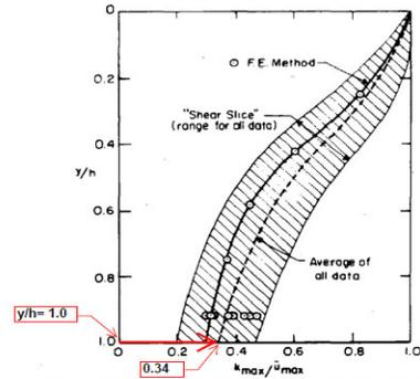
FIG. 9 VARIATION OF "MAXIMUM ACCELERATION RATIO" WITH DEPTH OF SLIDING MASS
