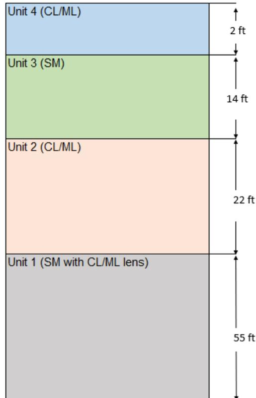
**Figure 2 Subsurface Stratigraphy**
