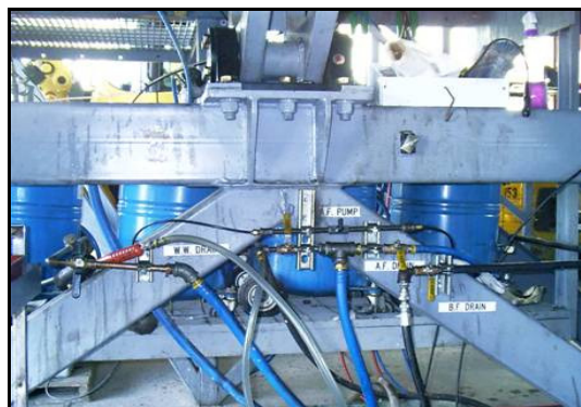
Vehicle fluids are then contained in dedicated recovery tanks.
