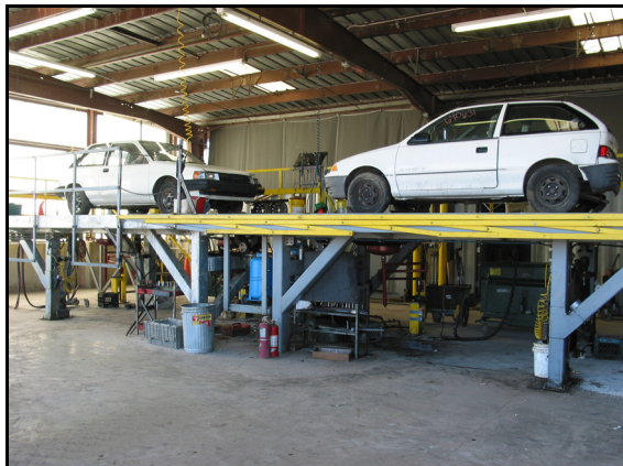
Two vehicle rotating drainage rack system with built-in fluid extraction system.
