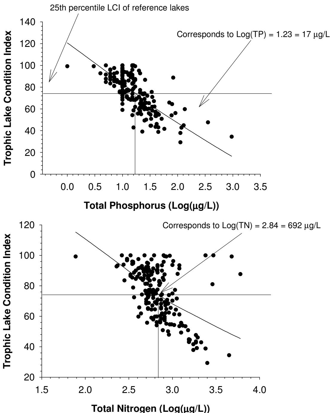
**Figure 7. Loess regression plots of total phosphorus and nitrogen against the trophic lake condition index (tLCI) in alkaline color lakes.**
