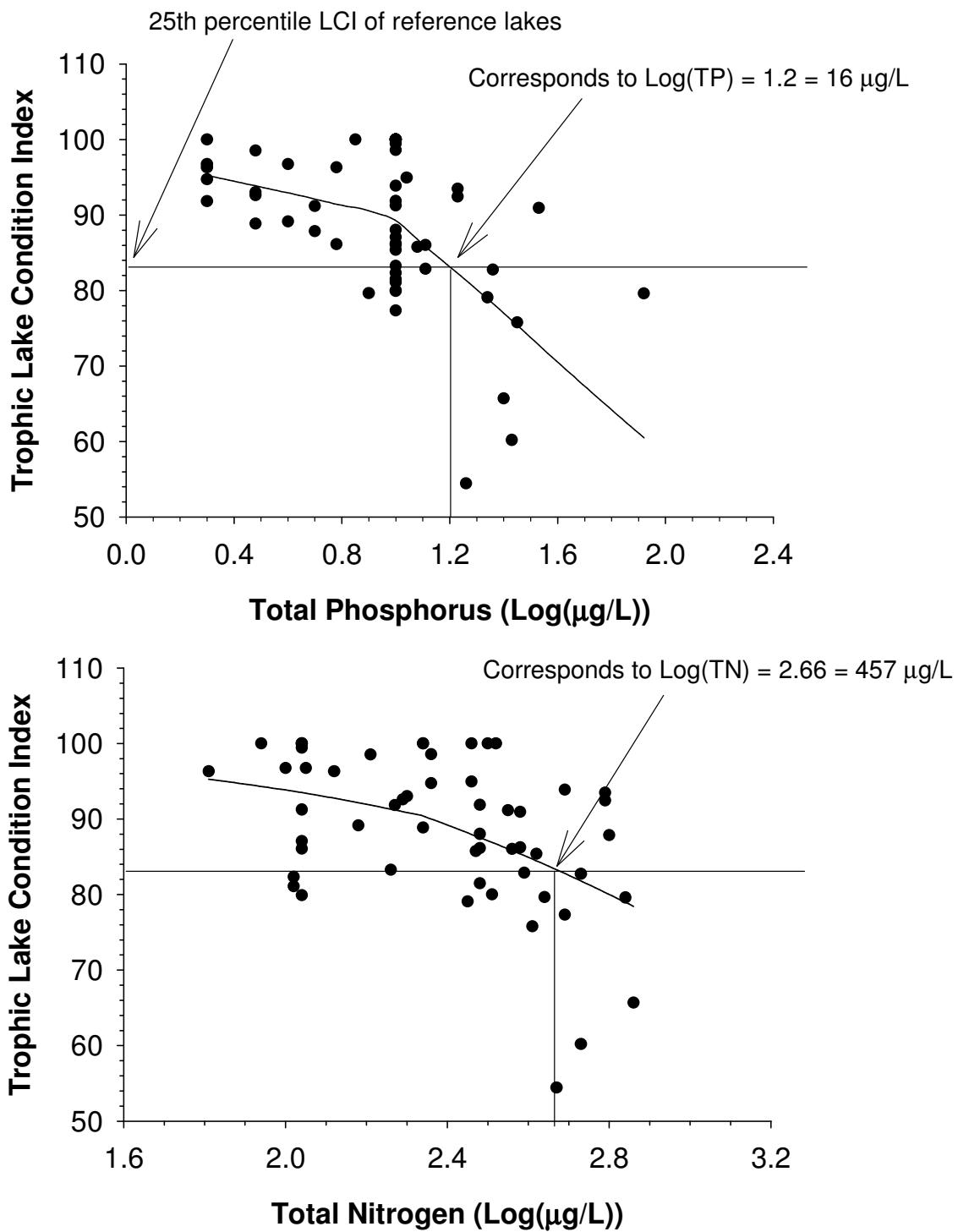
**Figure 4. Loess regression plots of total phosphorus and nitrogen against the trophic lake condition index (tLCI) in acid clear lakes in Region 75.**
