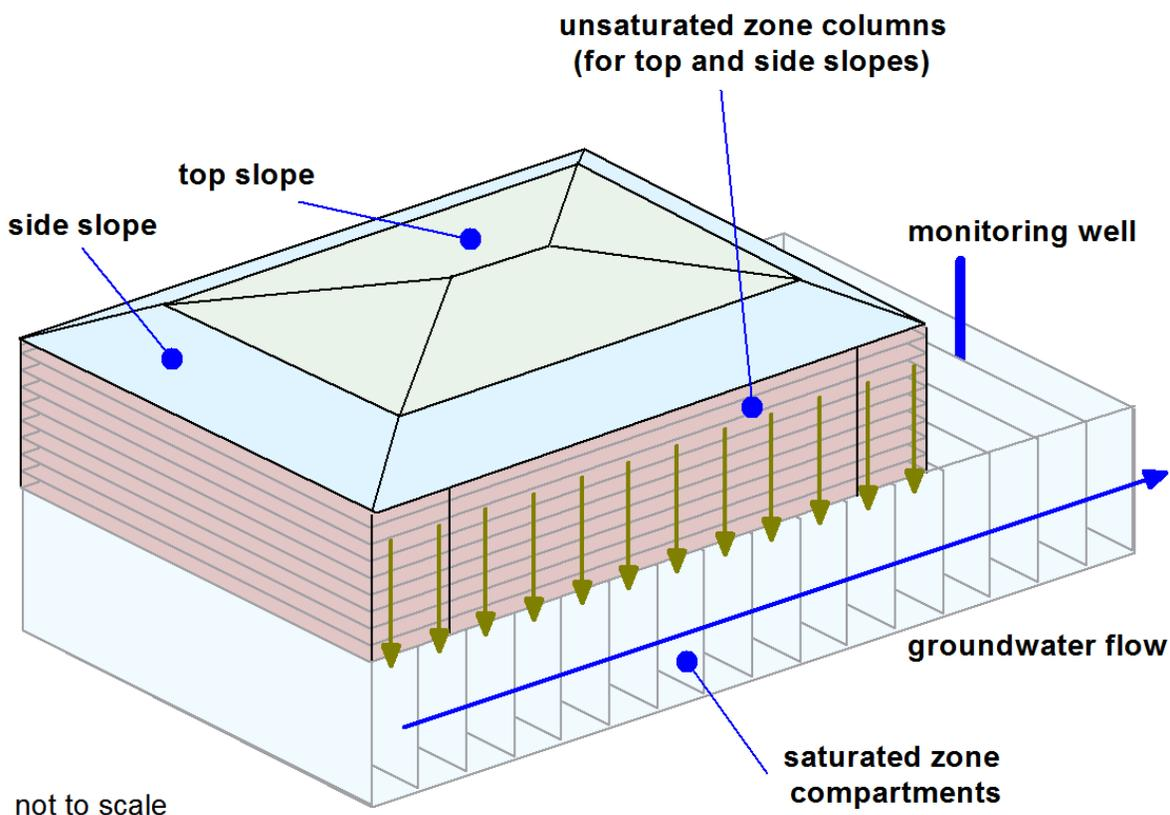
**Figure 2: Schematic representation of unsaturated zone and shallow aquifer transport using cell pathways; section parallel to groundwater flow direction.**
