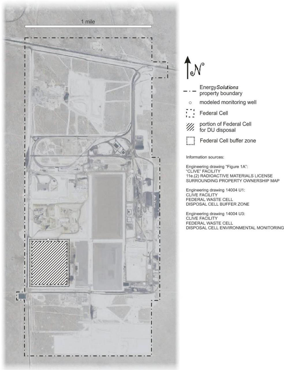
**Figure 1. Location and extent of the saturated zone modeling domain including location of the DU waste, the point of compliance monitoring well, the buffer zone of the DU cell, and outer boundaries of property owned and controlled by EnergySolutions.**
