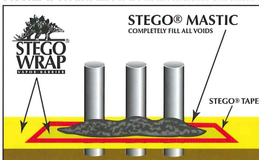
FIGURE 4: MULTIPLE PIPE PENETRATION SEALING
