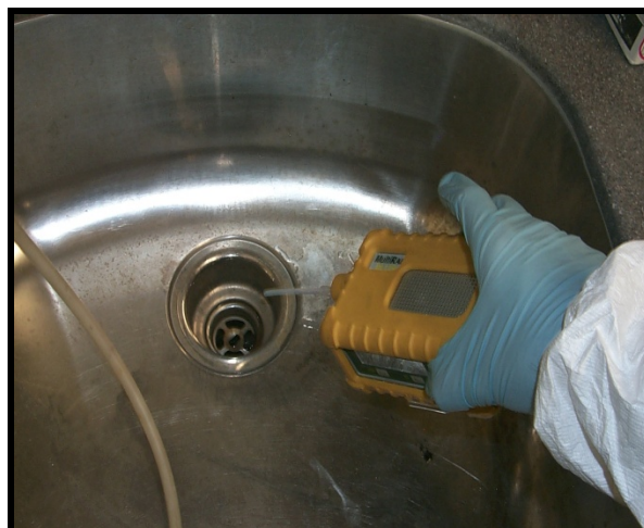
Testing a drain for volatile organics with a Photo Ionization Detector.
