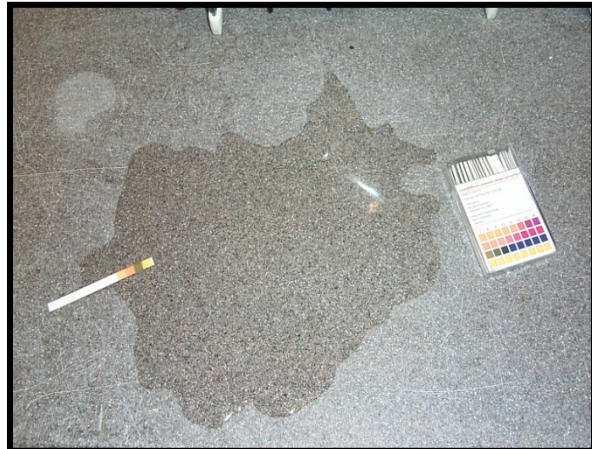
Testing a liquid encountered on a surface with a pH test strip.
