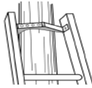
Ladder with a single support attachment for a pole
