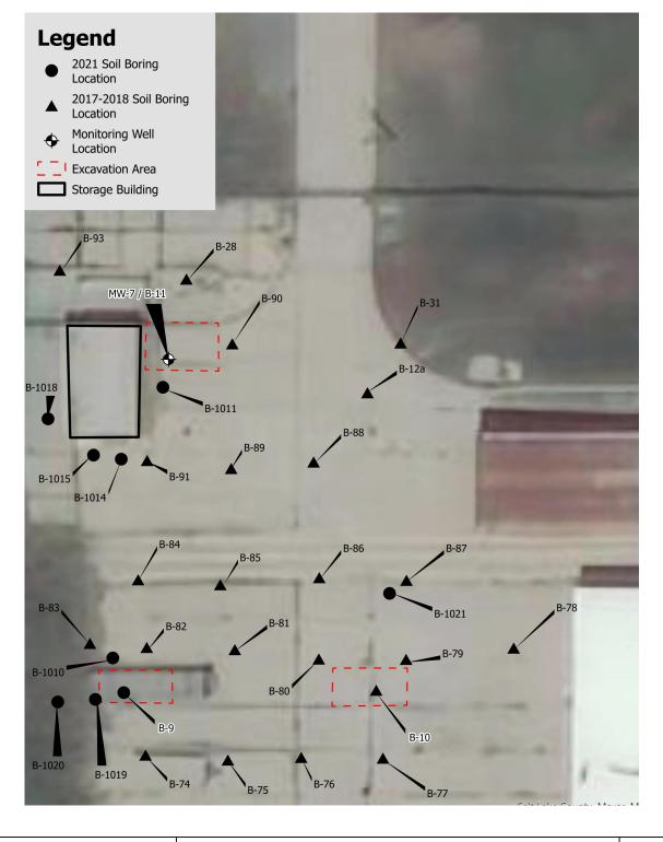
SCALE CLIENT PROJECT NTS **GENERAL ELECTRIC GENERAL ELECTRIC** 2022 REMEDIAL ACTION PLAN DATUM / PROJECTION 130 EAST 1100 NORTH NORTH SALT LAKE, UTAH 84054 CHKD BY DATE TITLE FIGURE WSP USA ENVIRONMENT & LOADING DOCK 10/07/2022 INFRASTRUCTURE SOLUTIONS INC **EXCAVATION AREA** PROJ NO. 216 CENTERVIEW DRIVE, SUITE 300 BRENTWOOD, TN 37027 DWN BY 4 WDP0014
