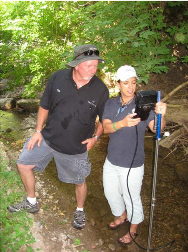
Hilary and Tim Rose with Salt Lake City Public Utilities measure in-stream flows to help determine the severity of water contamination.
