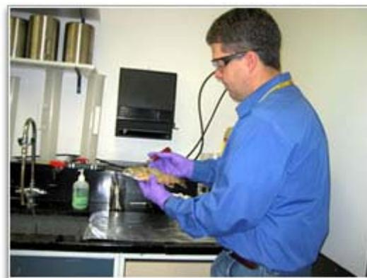
He removes a thumb-sized portion of the trout, peels off the skin and mashes the flesh in a crucible. The results are then placed in a sample tube that has been pre-screened to ensure that it is free of mercury or any other contamination that could compromise the results.
