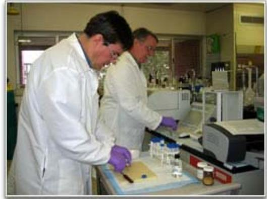
At the state health laboratory, scientists Steven Butala and Larry Scanlan take the sample tubes prepared by English and Brown and begin another round of preparations for analysis. Dr. Butala removes a sample from the tube and places it on a cutting board that has been sanitized overnight in acid and cleaned with ultra-pure water.
