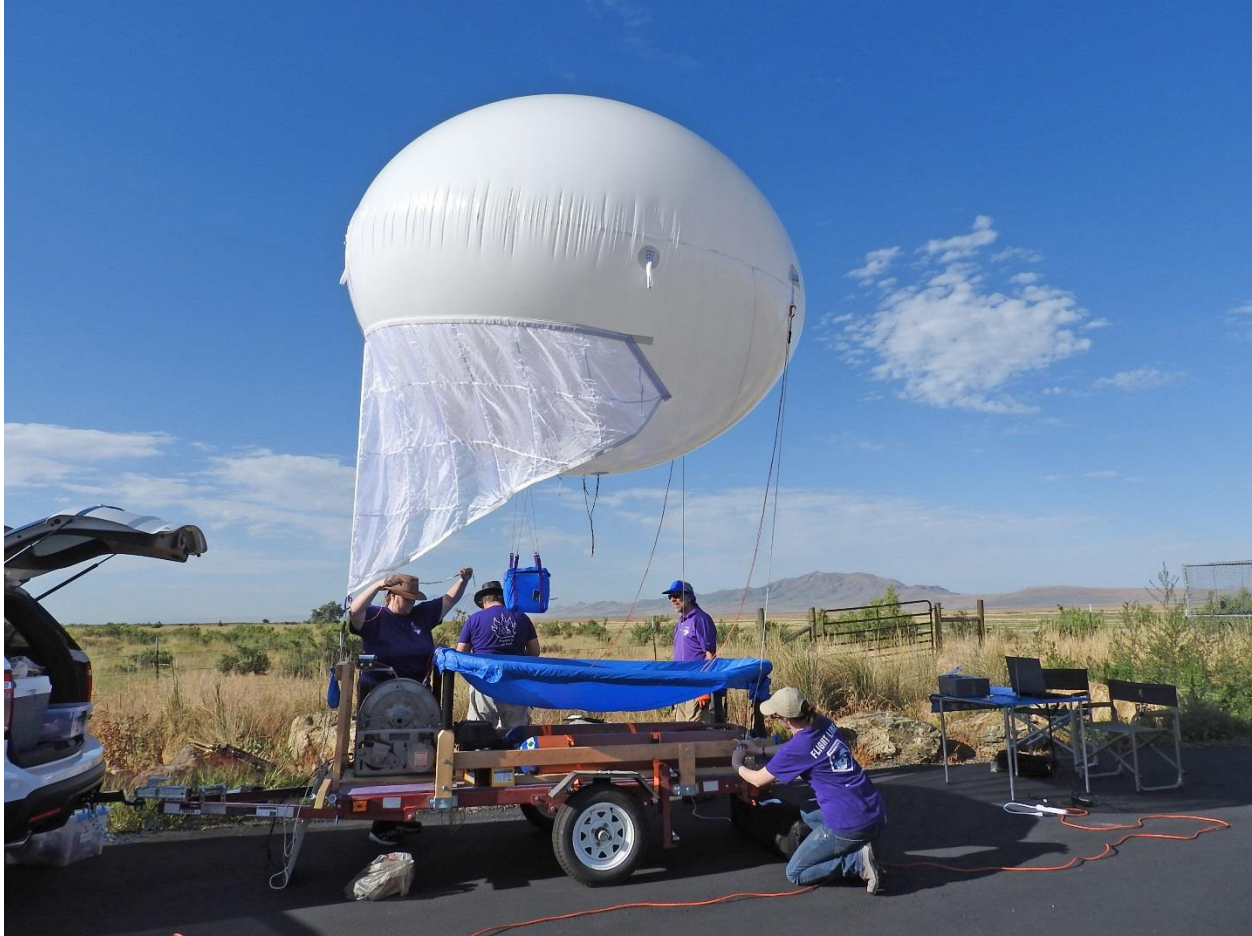
Figure B3. The entire tethered sonde system showing the support trailer with the mooring line winch on the front of the trailer.
