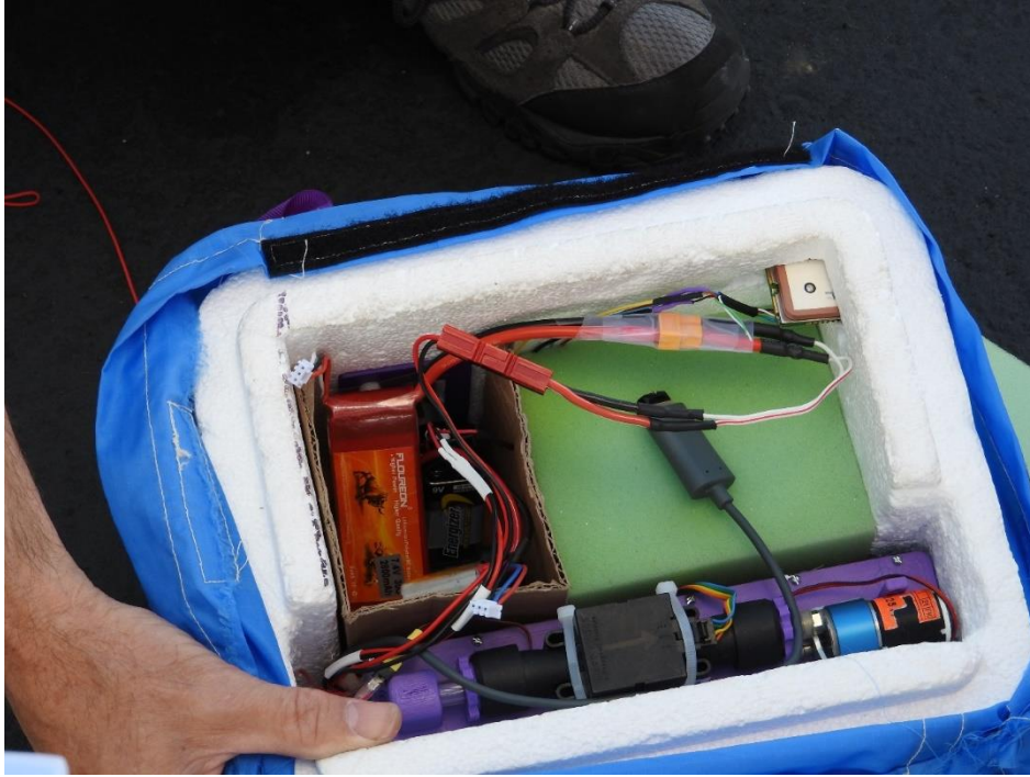
Figure B4. The AtmoSniffer and support equipment is mounted inside a foam protective box. This is version 1.0, the next version (1.1) is currently being constructed and will be significantly more compact.
