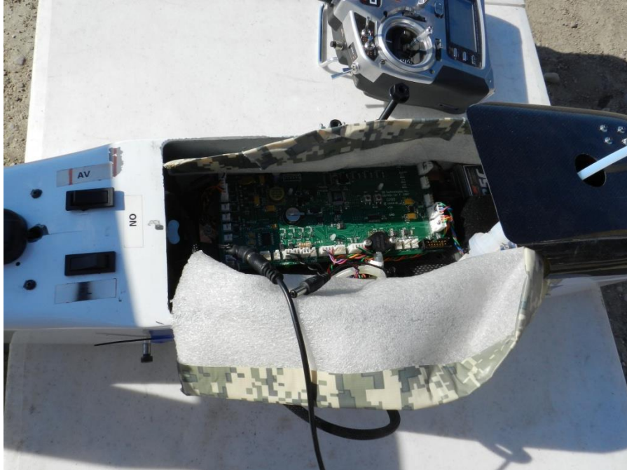
Figure 6. The modified O 3 monitor mounted in the UAV's payload bay.
