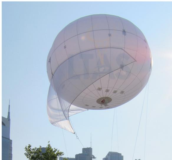
**Figure 1. Kingfisher aerostat. The model being used for these measurements is 8 feet in diameter and 7 feet tall with a 1.5 to 2kg payload capacity.**
