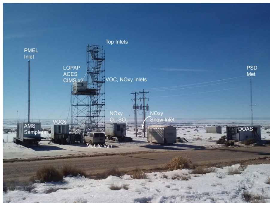
Figure 4-1. The Horsepool measurement site as configured during the 2014 intensive study.
