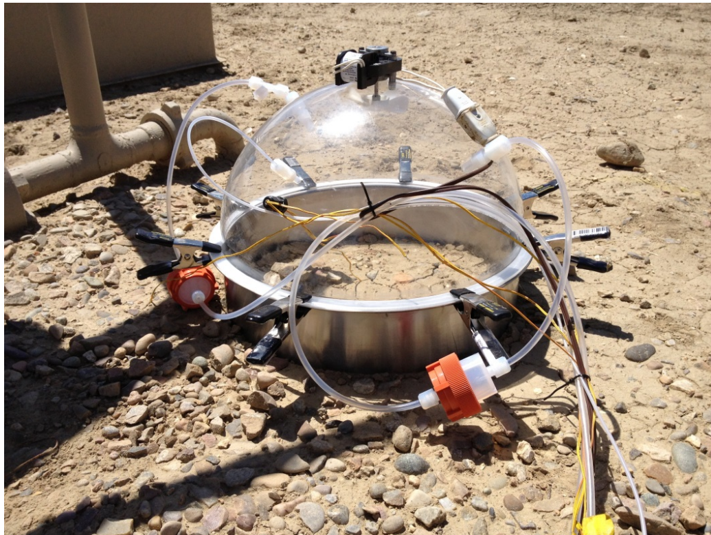
Figure 5-6. USU flux chamber samples soil emissions at a well site in Utah.
