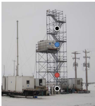
Figure 4-16. Tower used for sampling during the UBWOS 2014 intensive study at the Horsepool site. The indicated sampling levels were 1m, 3m, 7m and 14m agl.
