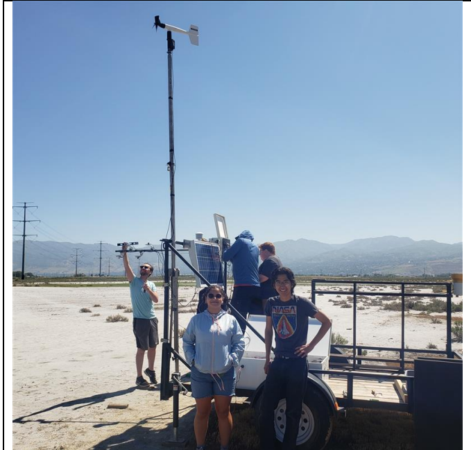
Figure 9. Weather, radiation, and ozone sensors deployed with up/down pairs of radiation sensors viewing a playa surface within the wetlands of Farmington Bay. Sodar, USDR5, was located nearby. Undergraduates Alejandra Garcia, Sam Jurado (foreground), undergraduate Nicholas Buckley (left), staff Colin Johnson and graduate student Aaron McCutchan (background).
