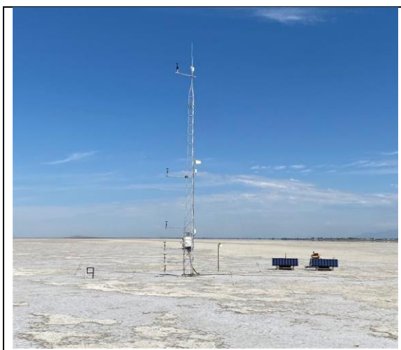
Figure 13. UUPYA tower on the Farmington Bay playa. Ozone and extensive meteorological sensors mounted on the tower.
