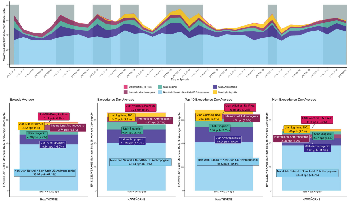
1 2 Figure 21: Source contributions by region and emission sector MDA8 ozone concentration (ppb) at the Hawthorne monitoring 3 station for each day of the modeling episode (upper panel) and on average over all days of the modeling episode, exceedance 4 days, top 10 exceedance days and non-exceedance days (lower panel). Results are based on 2023 OSAT model outputs for the 5 1.33 km modeling domain and spin-up days are excluded.
